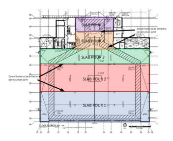
While this plan for placing the slabs certainly saves some time by eliminating the number of construction joints with dowels, it created many headaches for the project team when it came to determining effective finishing methods. The 75 feet sections are much wider than most slab pours that Kinsley Construction typically deals with on other projects. To complete the process, some of the intended finishing techniques must be modified and potentially compromised.
